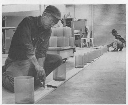
MASS PRODUCTION of the special luminarias for Bldg. 800 decoration is shown above. In the foreground Silas Shane (4511) works on an electrical connection while Reynel Garcia (4513) attaches lights to the wooden base in background for waterproof luminarias.
